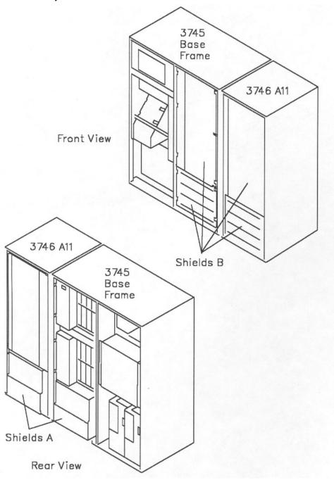
2. Open the internal shields B.
